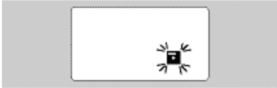
The torque wrench memory is full. Further bolting processes can be carried out, but these will no longer be saved.
