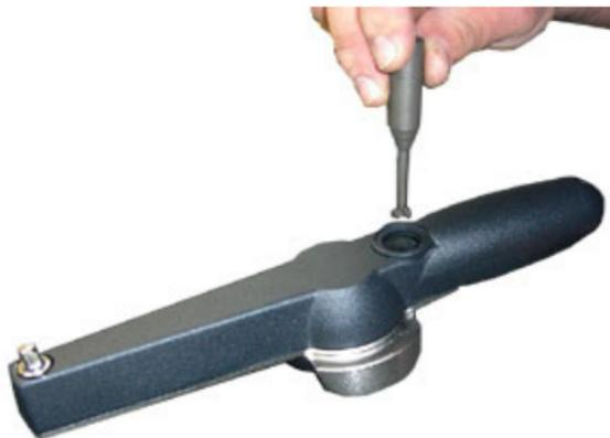
Make sure the movement arm is in-line with the wrench centerline. If the pushrod is off to one side the wrench may not calibrate in one direction or the other (see Fig. 5 and 6 below). The pushrod must also be perpendicular to the top plate or non-linear results may occur (Fig. 7).
